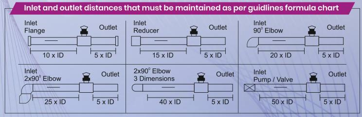
Note: • In Vertical piping only Upstream flow is recommended
